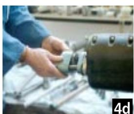
After carrying out operations 1(a) through 4(d) drive piston out of cylinder towards nearest end using a suitable steel drift and hammer.
